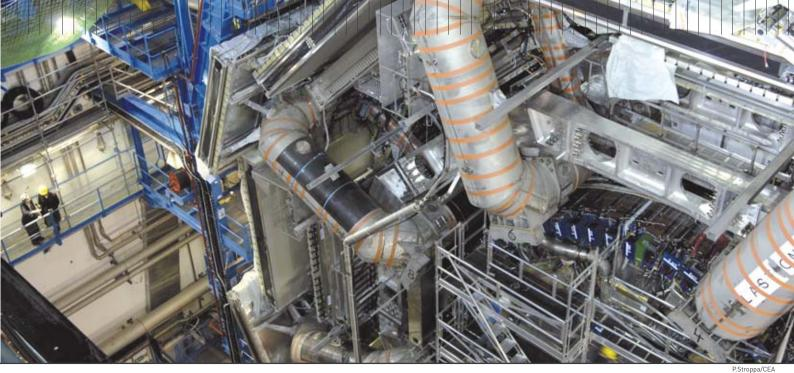
View of Atlas, one of the detectors installed at the Large Hadron Collider (LHC) due to come into service in 2008 at the CERN near Geneva. Four of the eight toroidal superconducting coil magnets in the facility are partly visible. The CEA is contributing to the design of this detector, together with that of the compact muon spectrometer (CMS).
